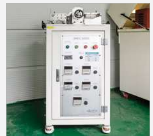
Room temperature torsion spring durability tester
